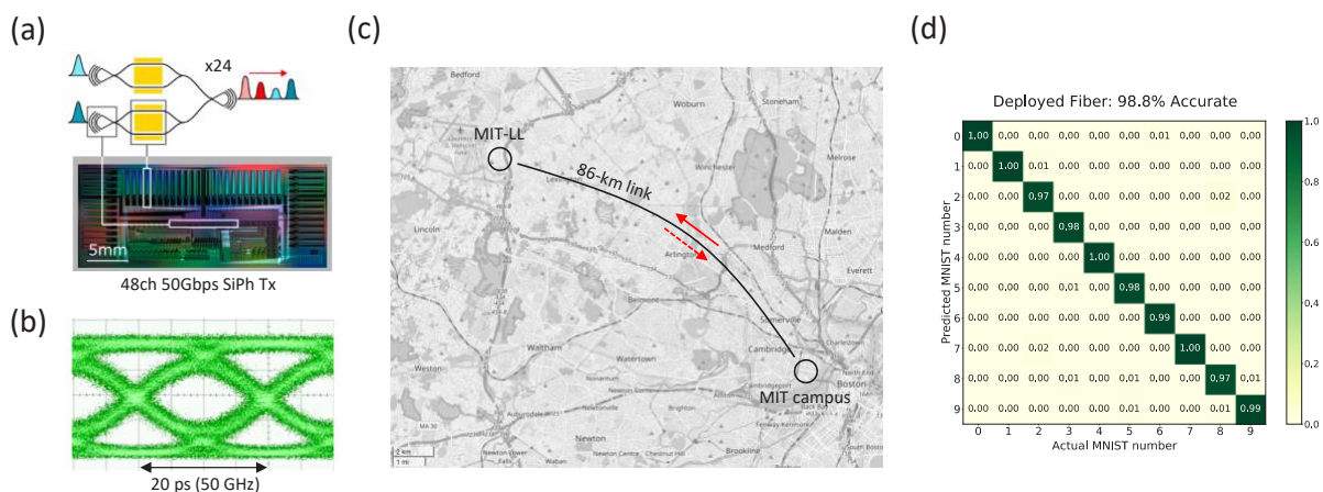
Fig. 2. Experimental demonstration of NetCast. (a) SiPh smart transceiver used as a weight server. (b) Eye diagram showing 50 Gbps OOK transmission through a single MZM. (c) Trunk link consisting of 43km of deployed optical fiber between MIT campus and MIT-LL, for a round-trip distance of 86 km. (d) MNIST classification accuracy for weight delivery over the deployed fiber.
